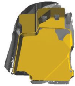
Nika Holding's CAD model of the scanned car floor.
