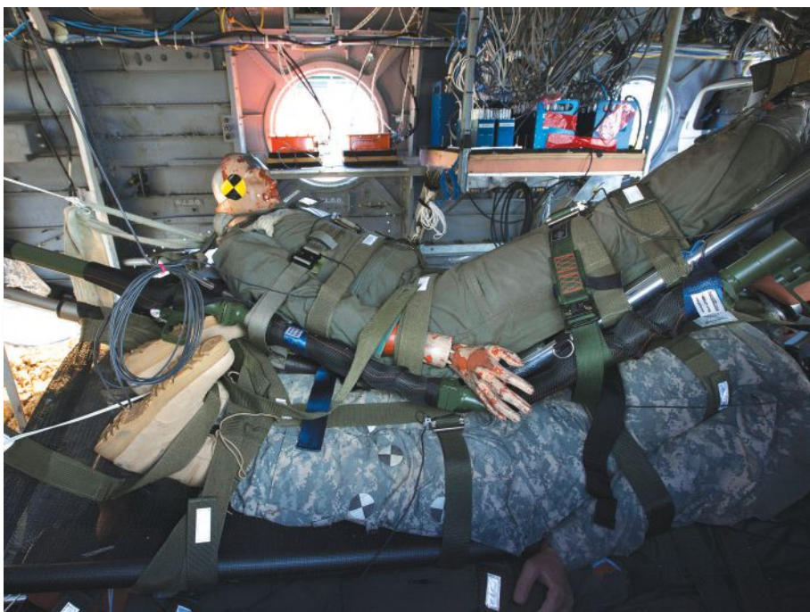
The manikin representing a real passenger in the drop test is wired with DTS data recorders that can withstand up to 500g shock. Image courtesy of DTS.
